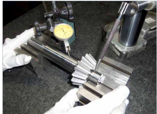
Concentricity test with dial indicator.
