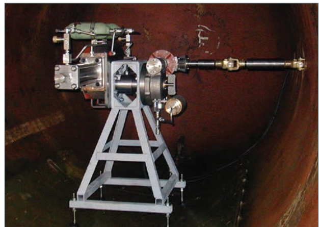
Hydrostatic qualification for subsea gearbox.
