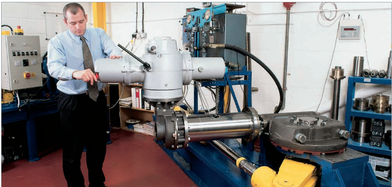
Endurance testing of prototype subsea gearbox.
