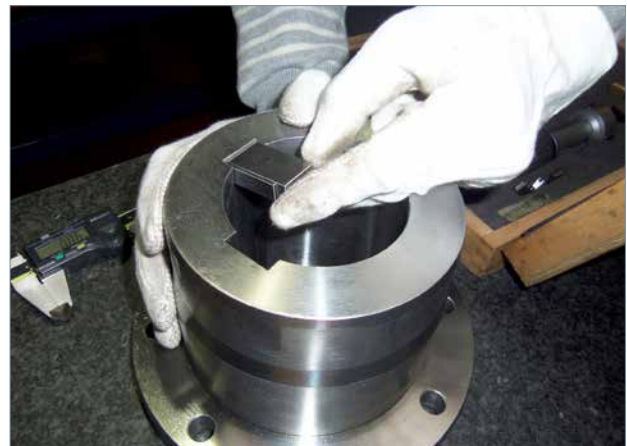
Bore and Key dimension check with gauge blocks.
